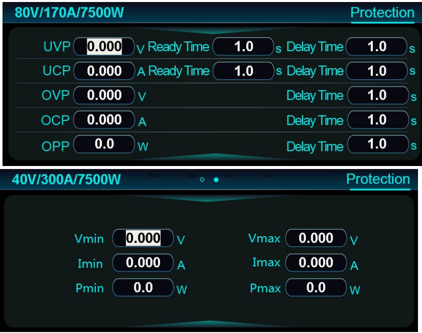
Figure 58 Protection Setting Interface
